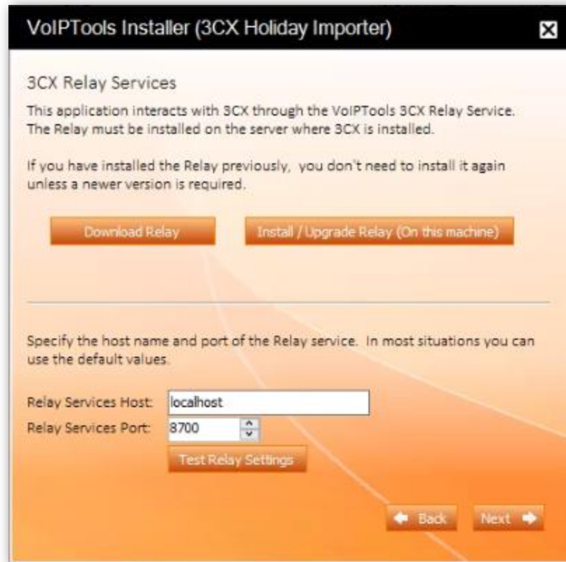
Figure 2: Test VoIP 3CX Relay settings
